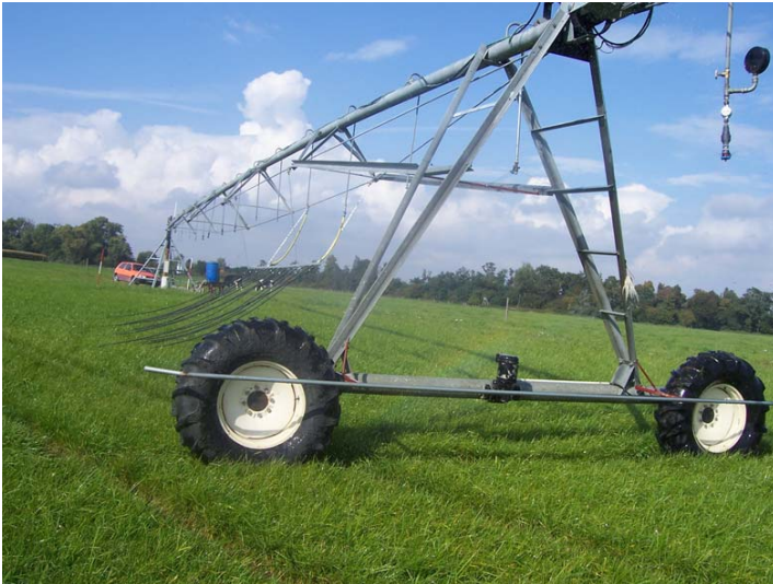
Appendix G: Installing a metallic bar parallel to CP wheel to avoid drop tube tangling in to mobile drip CP wheel
