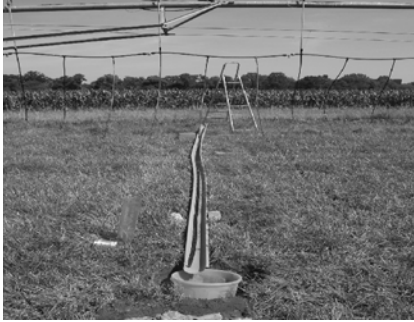
Figure 3.21: Field measurement of the drop tube water application rate
