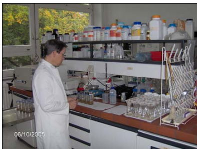
Measuring of pH (soil acidity) and EC (soil salinity)
