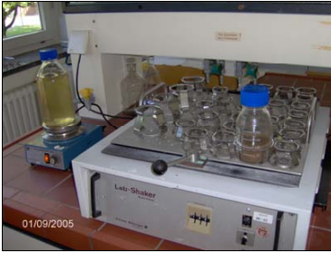
Shaking stage of soil samples
