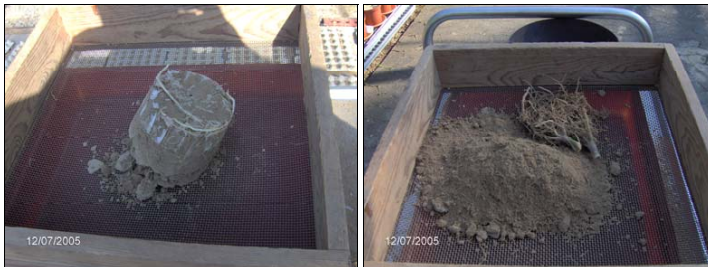
Put the soil including roots in sieve 2 mm and remove carefully the roots
