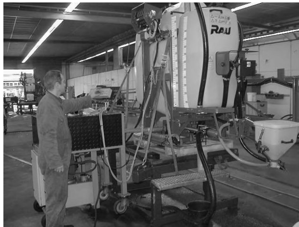
Figure 1 Inspection of a new sprayer comprises pump capacity, pulsations, leakages, safety valve and kinks
