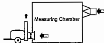
Arrangement for an one way sucking air-assisted sprayer in the measuring chamber
