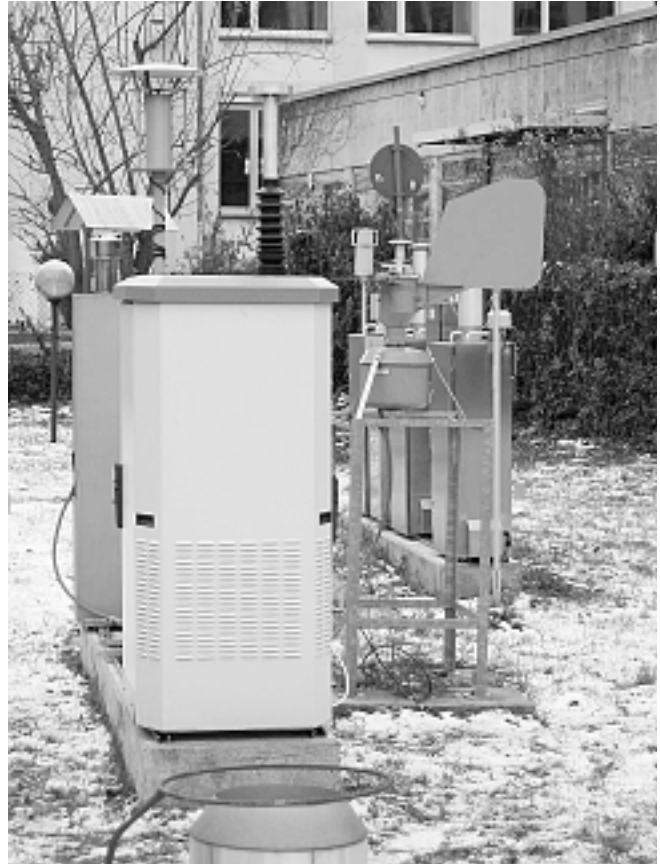
Fig. 10. Sampling site at the German weather service in Freiburg with the pollen monitor (left) and the Burkard sampler (right) for the field test 2006.
