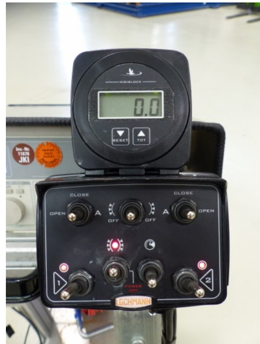
Fig.5: Pressure gauge and switchbox with switches for spray sections left/right /both and for moving the air cover shields.
