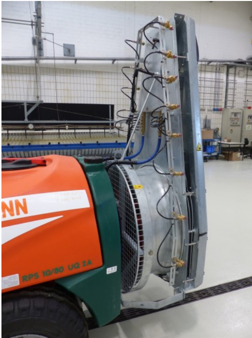
Fig.2: 800mm axial fan with air deflector device.
