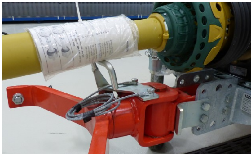
Fig.3: Rest for the PTO shaft so the coupling and front cardan joint don't touch the ground when it is uncoupled.
