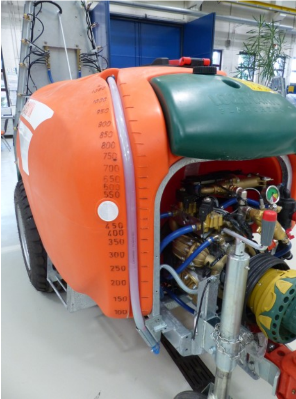
Fig.4: PTO driven pump and tank with contents indicator.
