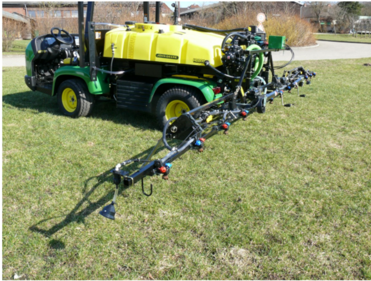
Fig.4: Carrier with mounted spraying unit with folded up support legs (between driver seat and tank), unfolded boom and foam marker
