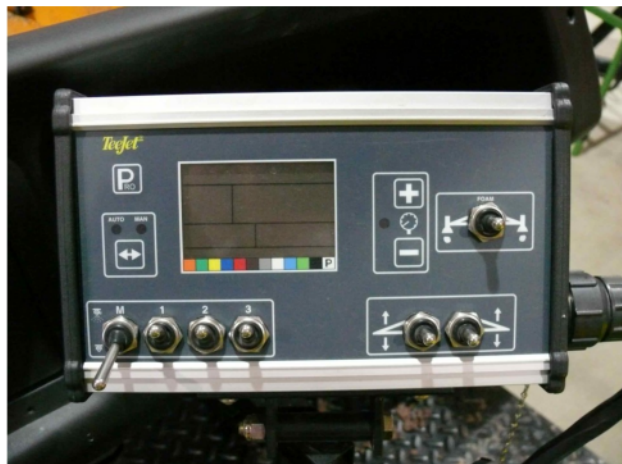
Fig.7: Spray computer, display and control panel near the driver's seat.
