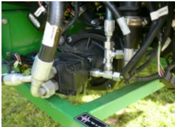
Fig.5: Hydraulic driven centrifugal pump.
