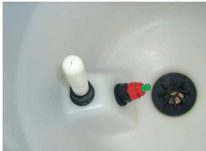
Fig.2: View to the bottom of the bowl. Rotating nozzle (white), mixing nozzle (green), suction opening with screen (black).
