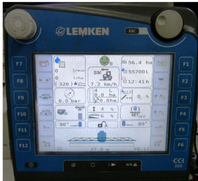
Fig.9: Lemken CCI 200 terminal in the driver's cab.
