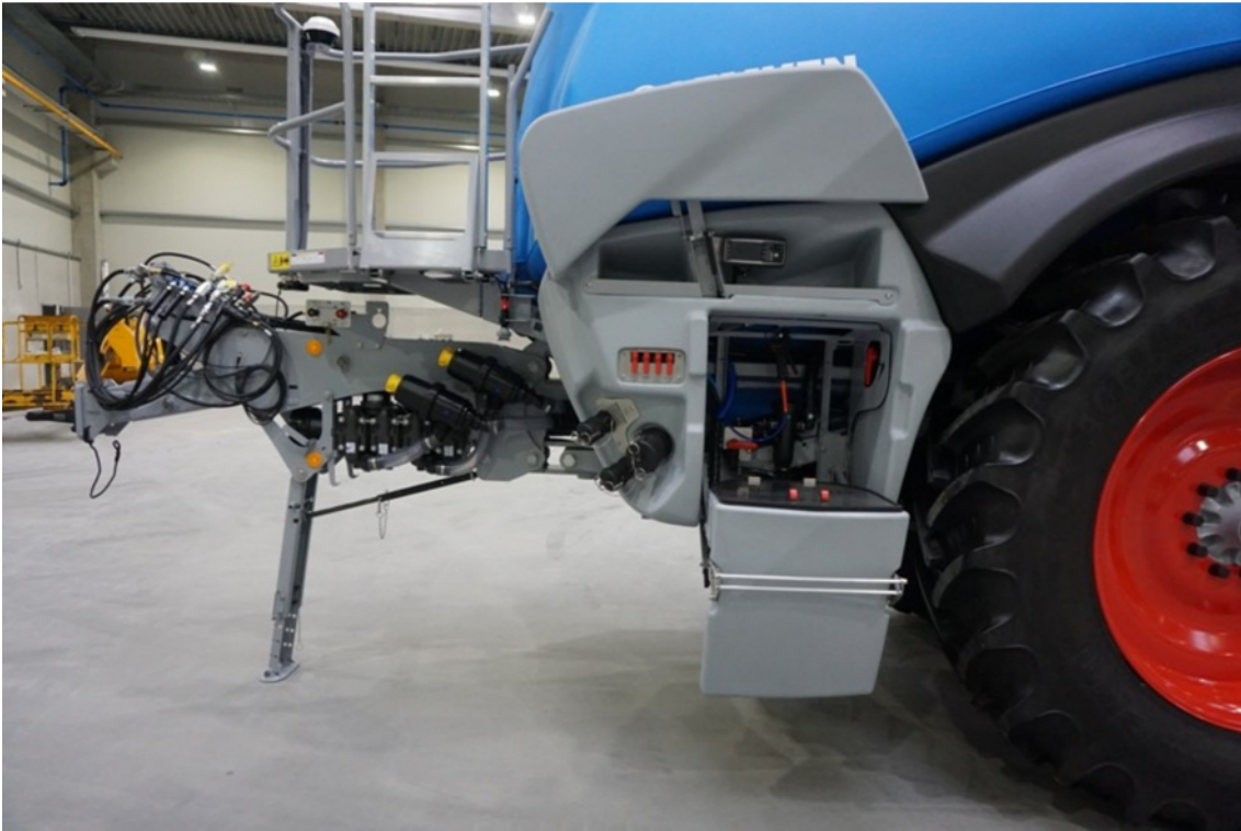
Fig.6: Left sprayer side with improved induction bowl and operating panel (above and left of induction bowl). With filling connections (left of the induction bowl).
