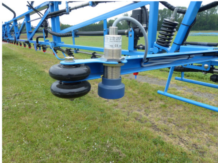
Fig.3: Boom with ultrasonic sensor, nozzle protection bar and obstacle give away device.
