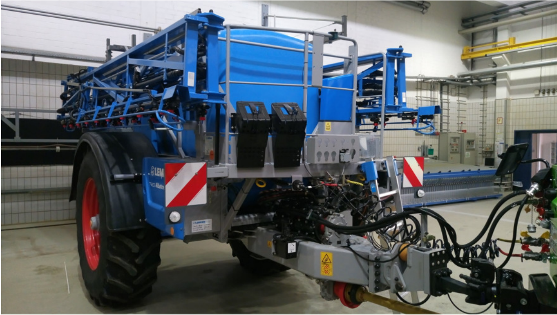
Fig.4: Sprayer with folded boom and steering drawbar with suspension (yellow plate).
