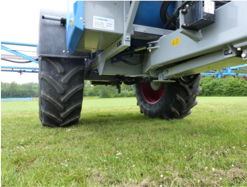
Fig.2: Frame with steering drawbar and parking support with hydraulic pump.
