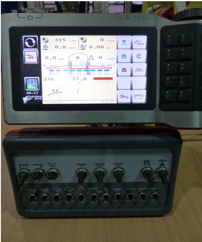
Fig.5: „ISO Match Tellus 60“ terminal (ISOBUS) with switch board.
