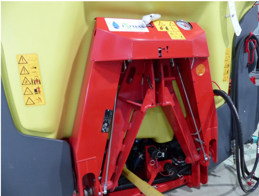
Fig.2: Quick coupling frame with analog pressure gauge.
