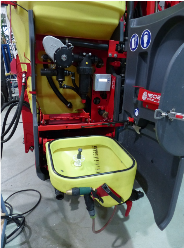
Fig.4: Left sprayer side with control centre and pulled out induction bowl.
