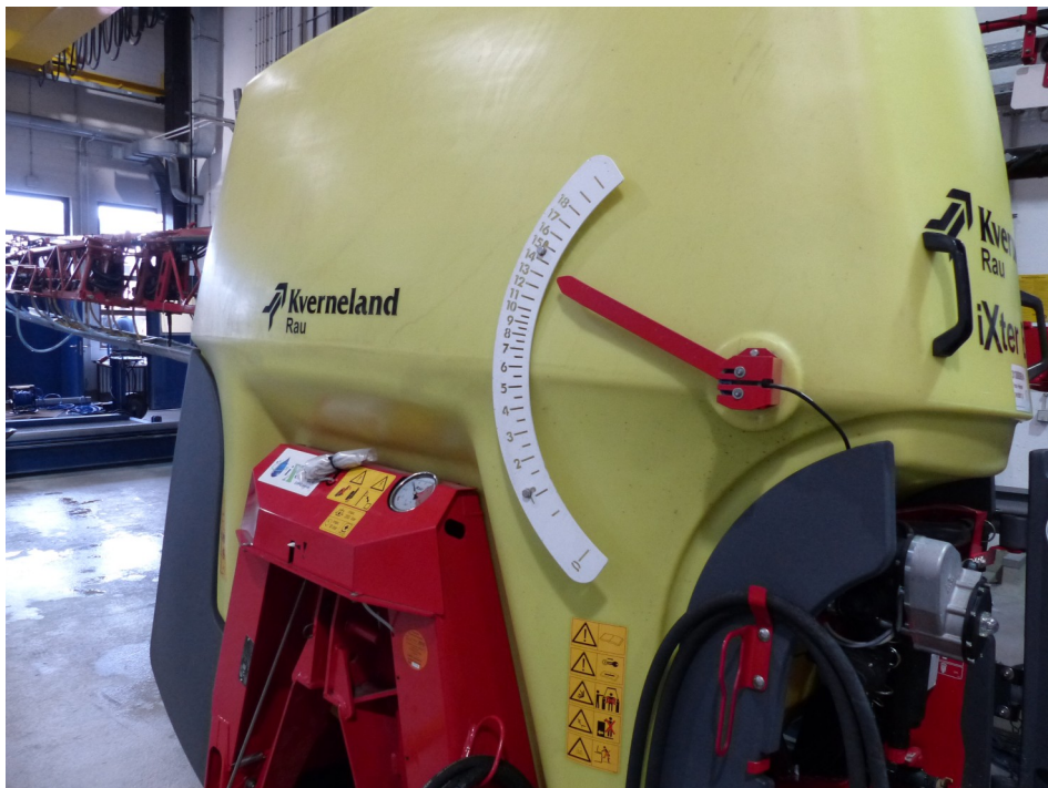
Fig.3: Contents indicator based on flush type fluid indicator.
