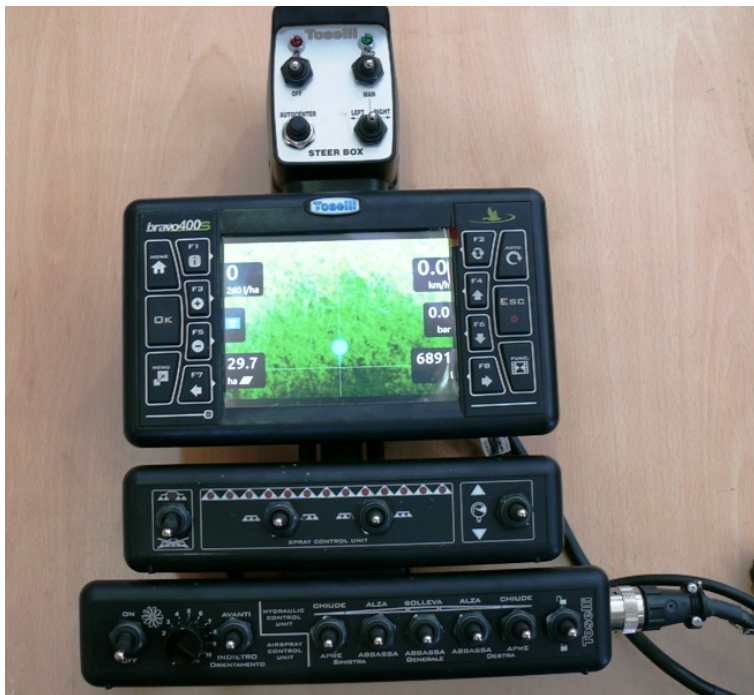
Fig.6: Spray computer terminal „bravo 400s“ with switchboards for operating the hydraulic, spraying and steering functions.
