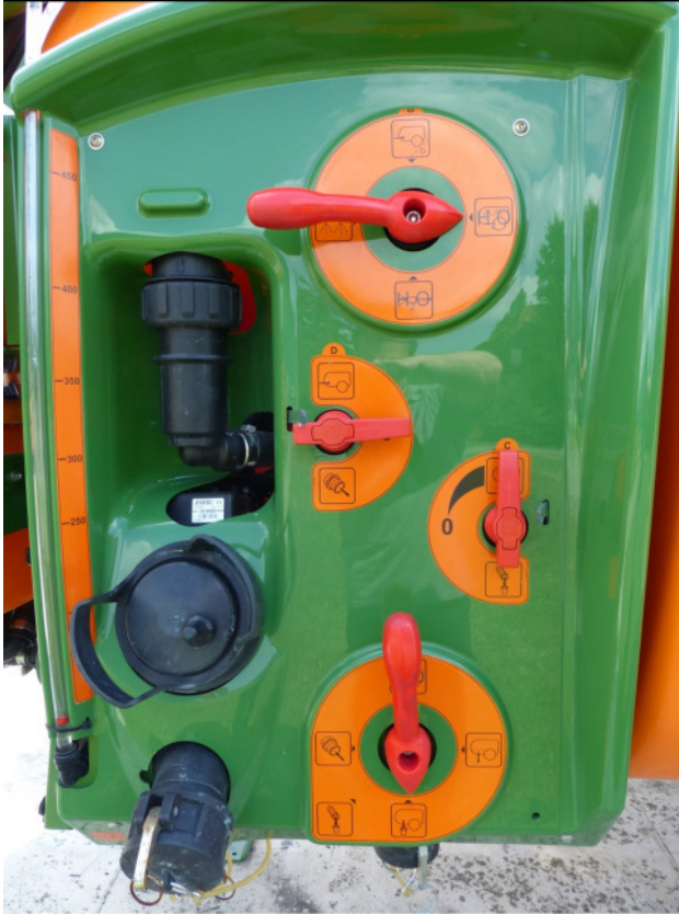
Fig.7: Left sprayer side with new operating panel, filling connections and contents indicator for rinsing water tank.
