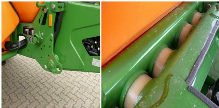
Fig.5/6: Mounting of the drawbar and shock absorbing PU-dampers.
