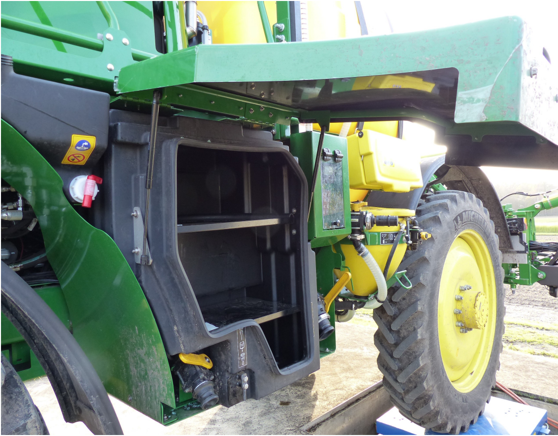
Fig.2: View of the left sprayer side with equipment box, control centre and induction bowl.
