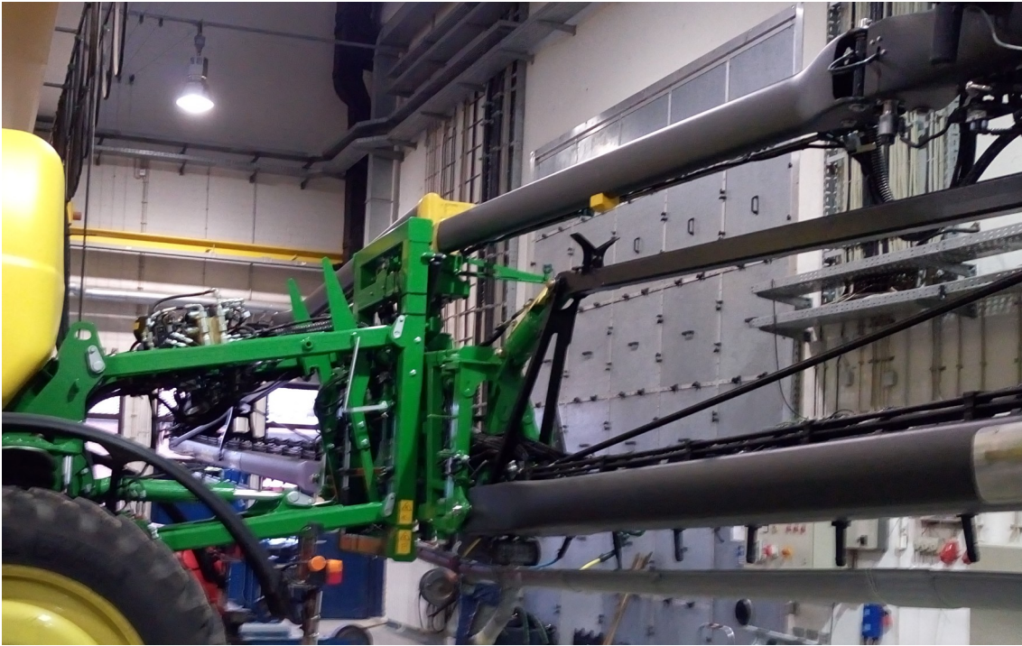
Fig.4: Boom lift for the lateral folding boom.
