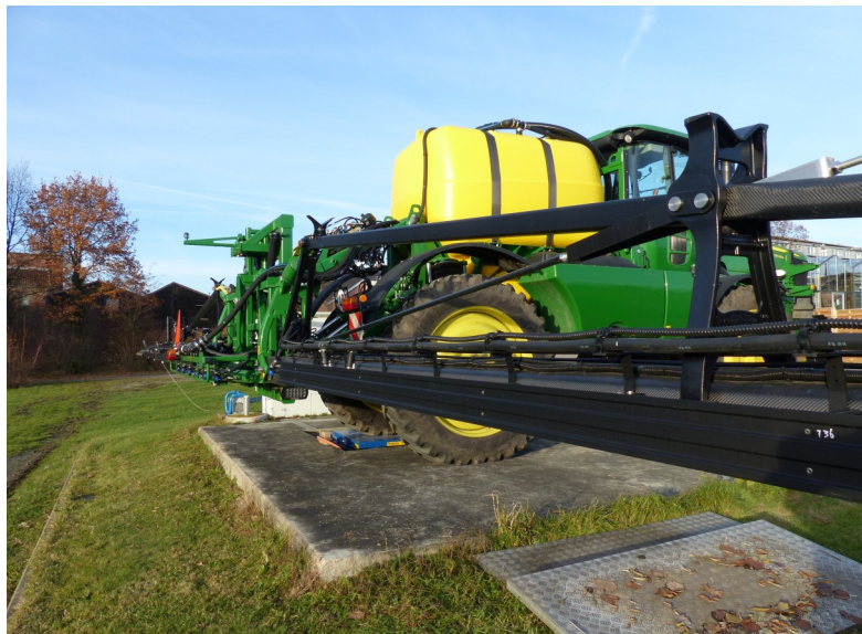
Fig.3: 36m steel / carbon fibre boom.
