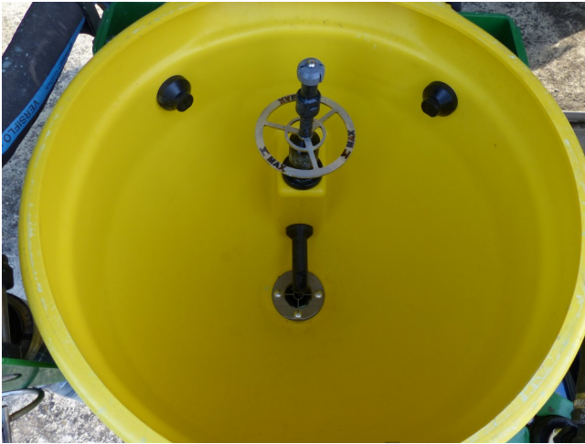
Fig.6: Induction bowl with rotating nozzle for can cleaning.
