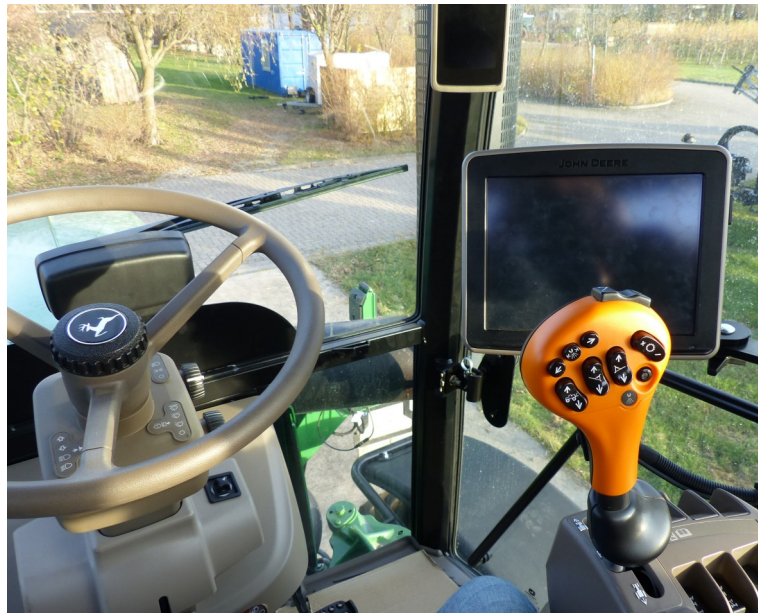
Fig.7: Drivers place with 10" touch-screen terminal and lever for steering of sprayer functions.
