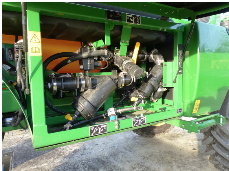
Fig.5: Right sprayer side: filters and filling connections.
