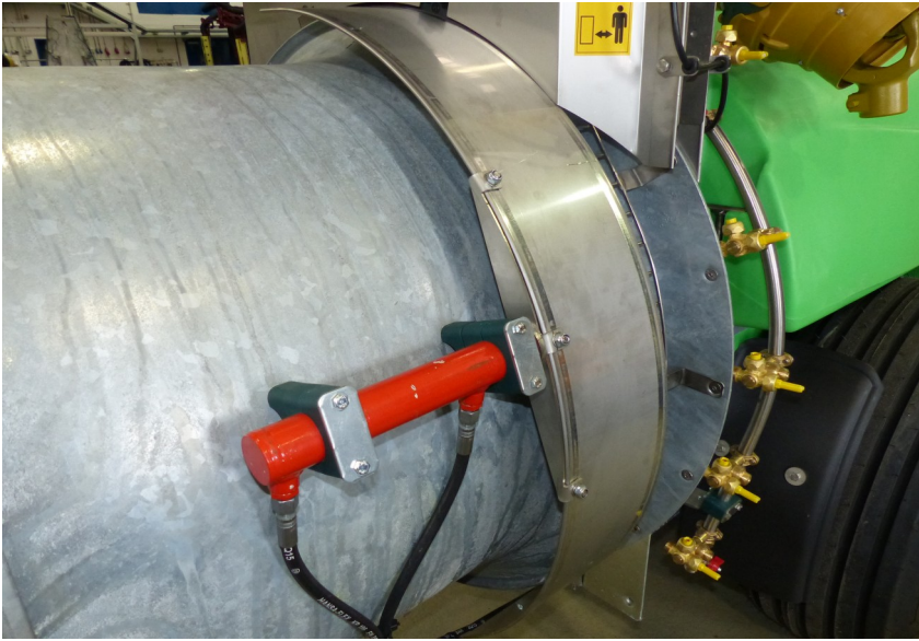
Fig.4: Hydraulic driven air deflector shield to reduce drift by avoiding the air stream support for this side.
