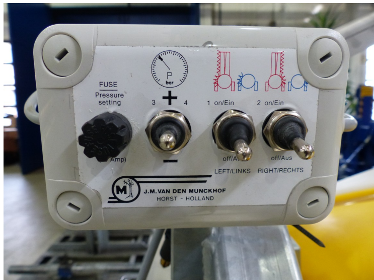
Fig.5: Control panel for pressure adjustment and nozzle section switching.
