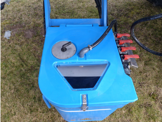
Fig.6: Induction bowl with contents indicator and rotating nozzle
