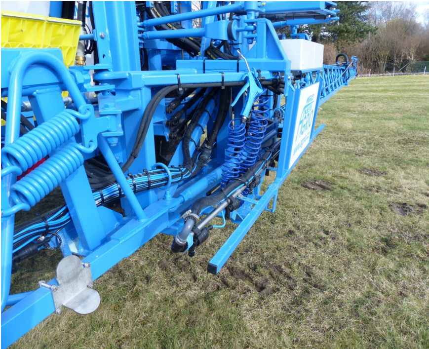
Fig.4: Central boom section with (steel rope) lift for the lateral folding boom.
