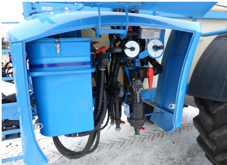
Fig.5: Left sprayer side: induction bowl, control center with filling connections.
