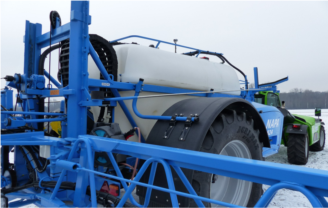
Fig.4: Steel rope boom lift for the lateral folding boom.
