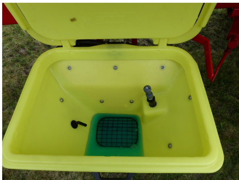
Fig.3: Open induction bowl on the left sprayer side.
