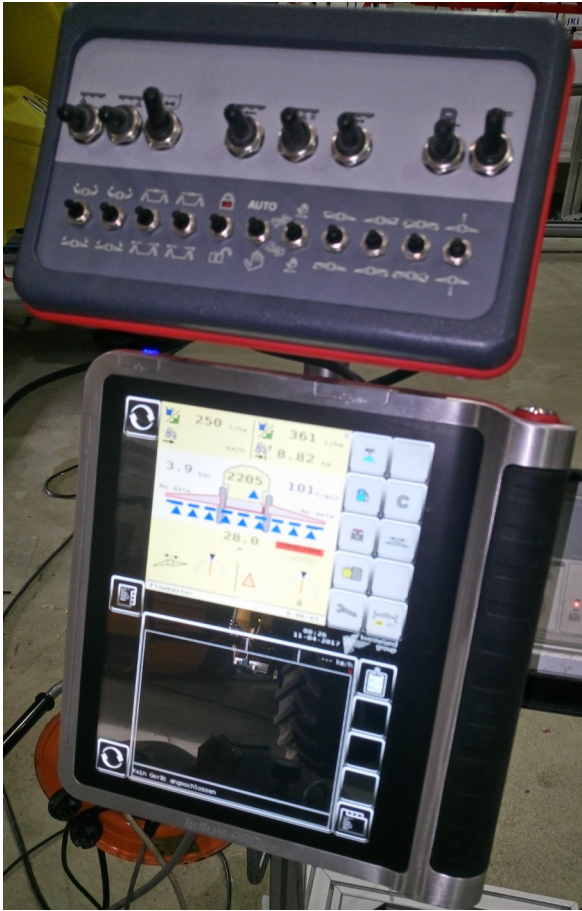
Fig.7: ISO match „Tellus PRO“ terminal (ISOBUS) with switch board.
