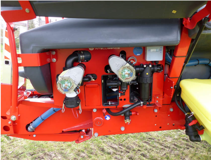
Fig.2: Control centre on the left sprayer side.
