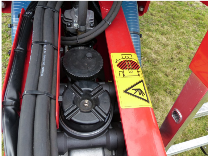
Fig.4: Two Altek P260 pumps placed in the drawbar.
