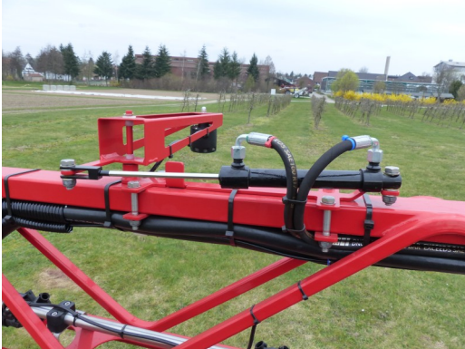
Fig.5/6: Independent bend of the boom arms. Ultrasonic sensor and hydraulic arm to swing ultrasonic sensor in parking position automatically whether the boom is folded.
