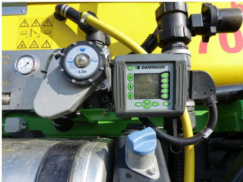
Fig.5: Control center on the left sprayer side.
