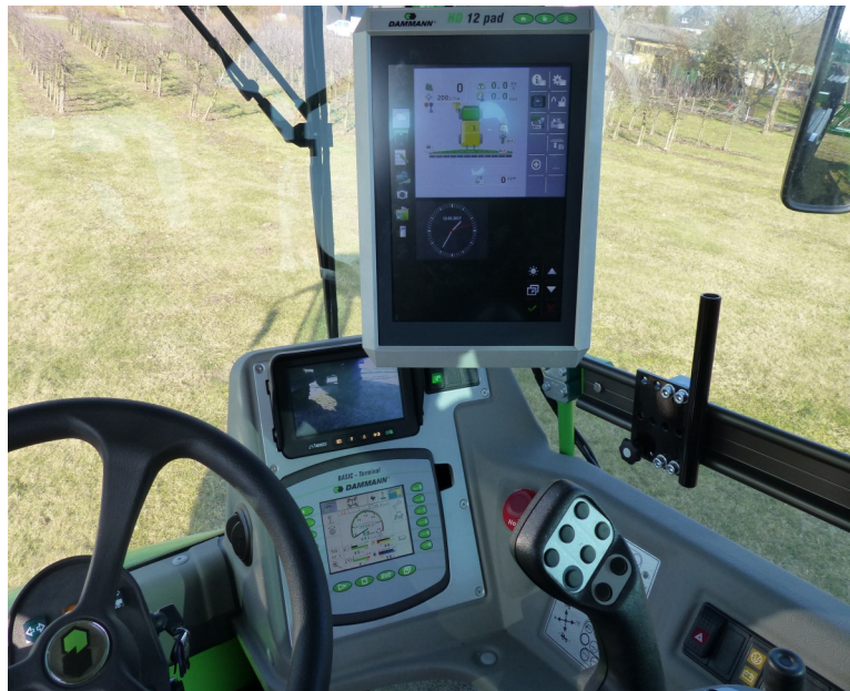
Fig.7: Drivers place with terminals for the driving and spraying functions (HD 12 pad). With monitor for the rear view camera (lower control panel).
