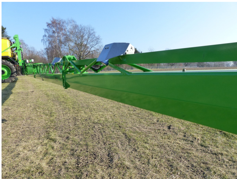
Fig.3: Steel boom with nozzle protecting lower boom profil and ultrasonic sensors for the automatic boom height control.
