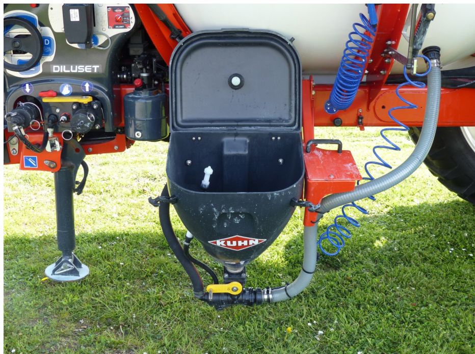
Fig.5: Left sprayer side with swung out induction bowl.
