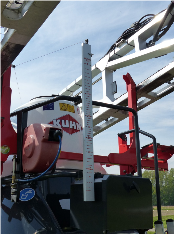
Fig.2: Front right view of sprayer with tank contents indicator and spray lance for outer sprayer cleaning.
