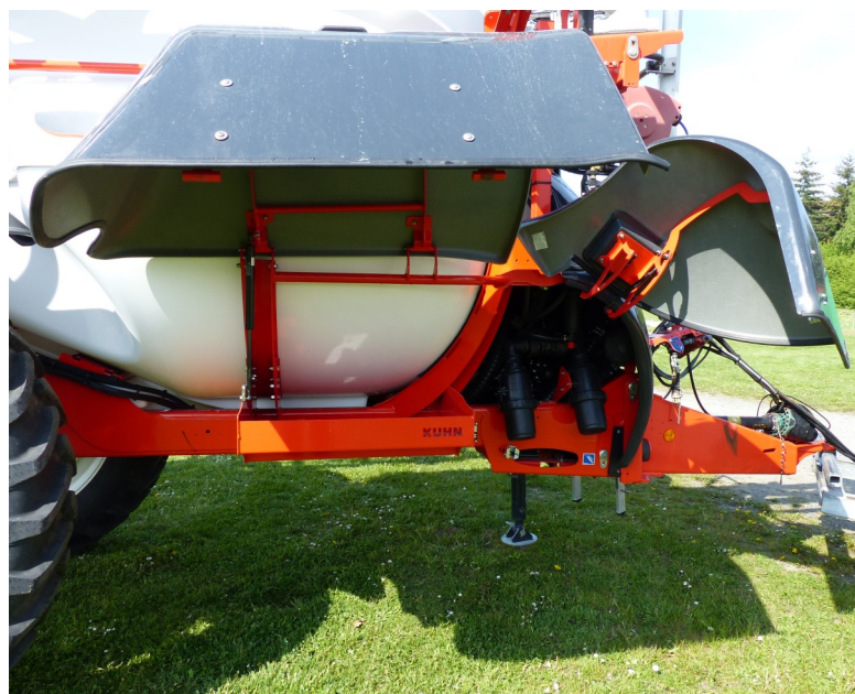
Fig.3: Right sprayer side with storage area and filters.
