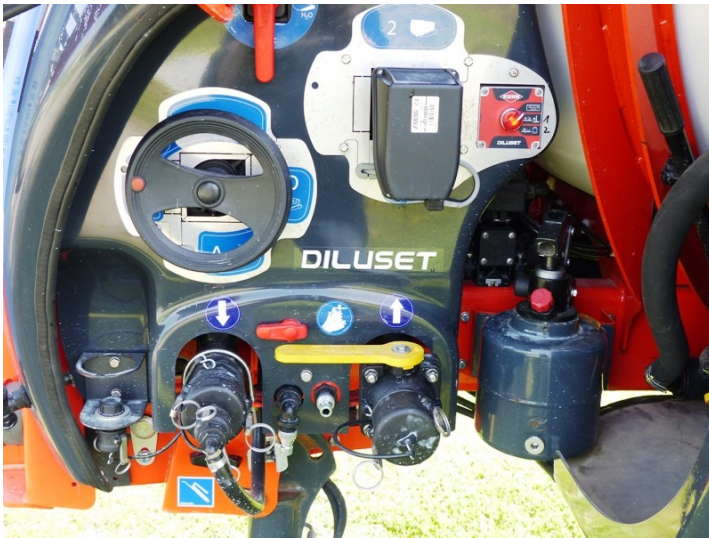
Fig.4: Control centre on the left sprayer side.
