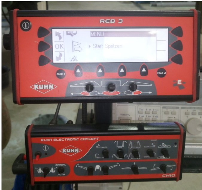
Fig.6: In the foreground: Display and controlboard (REB 3) and switchboard for the hydraulic functions (CH10) in the driver`s cabin.
