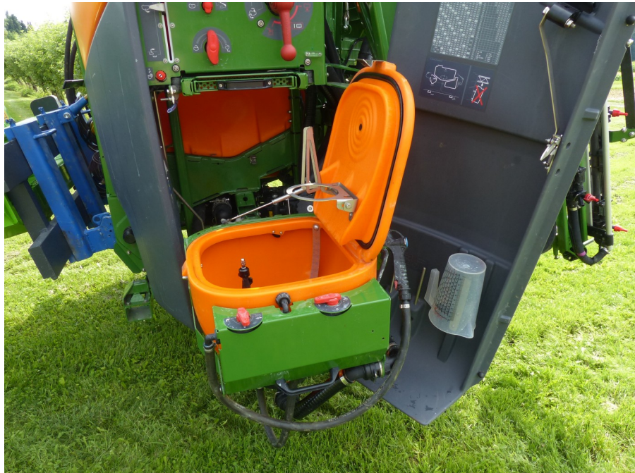
Fig.5: Left sprayer side: induction bowl and control center.
