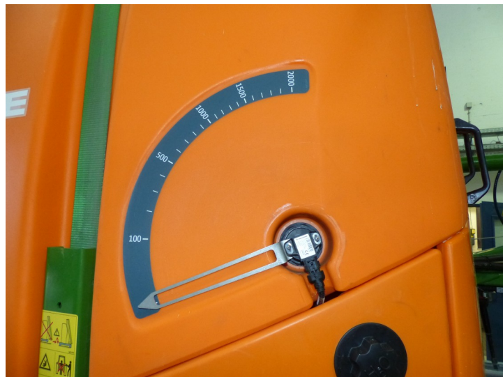
Fig.3: Level indicator with non-linear graduation.
