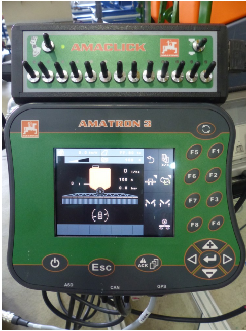
Fig.6: „AMATRON 3“ terminal and switchboard for displaying and controlling the spray and hydraulic functions.
