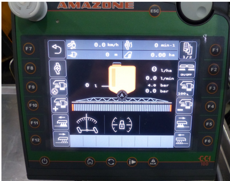
Fig.6: „AMATRON 3“ terminal with push buttons for displaying and controlling the spray and hydraulic functions.
