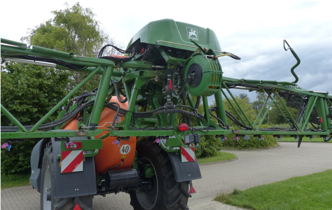
Fig.3: Lift and central section of the boom, with spray gun for cleaning and lights for visual spray control at night.
