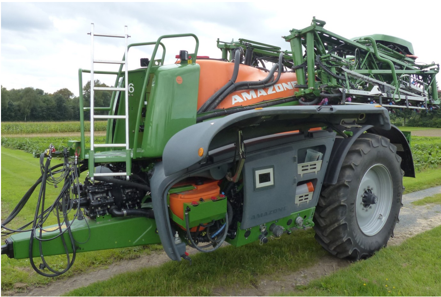
Fig.4: Left sprayer side: induction bowl, filling connections and control center with display.
