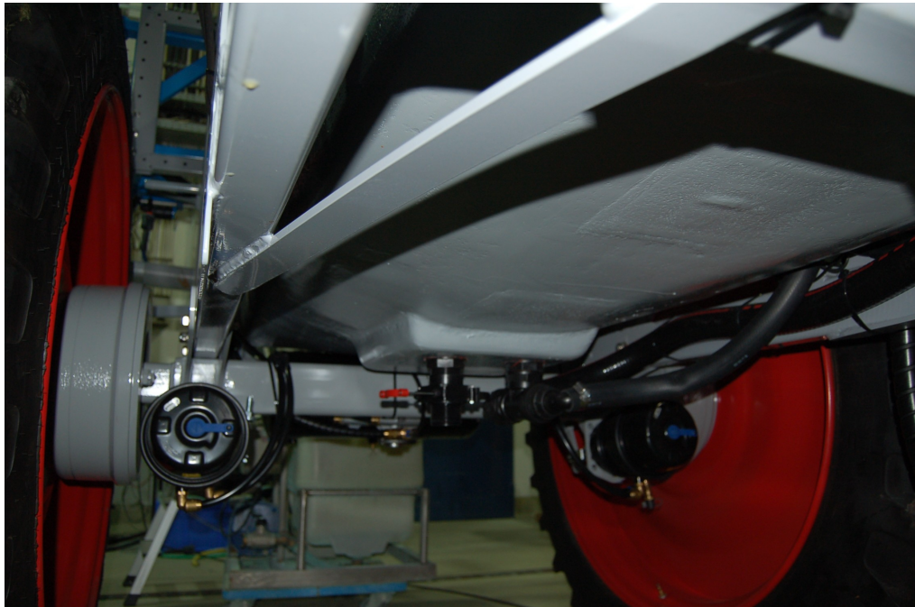
Fig.6: Rigid axle and flat tank bottom.
