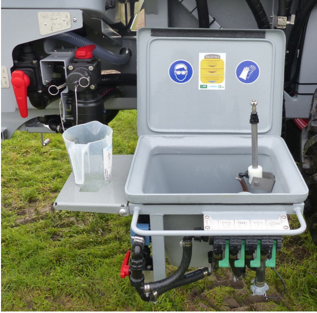
Fig.7: Induction bowl with erected rotating nozzle for can cleaning.
