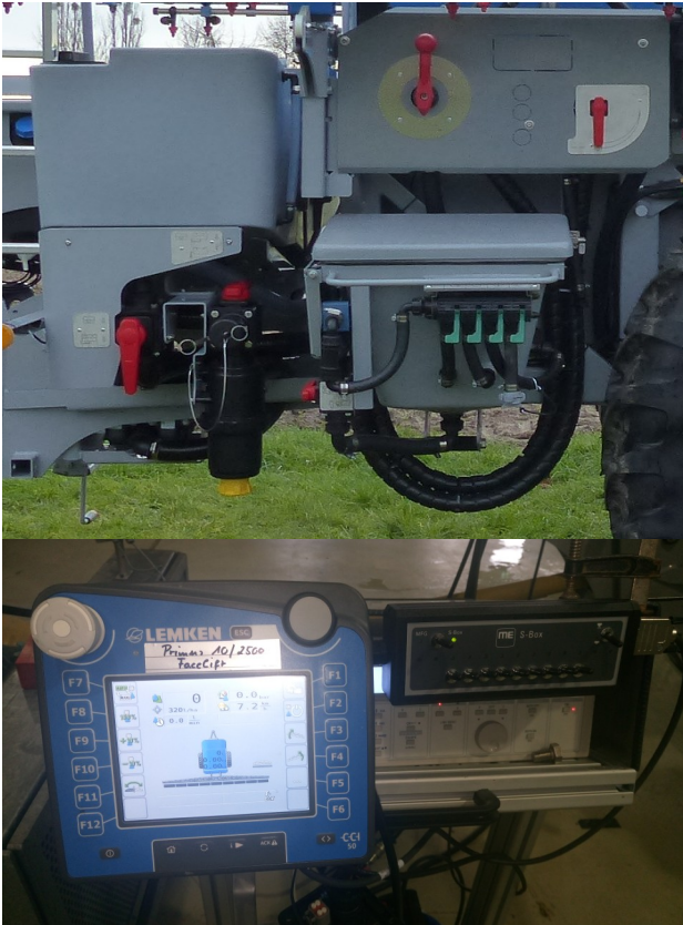
Fig.4/5: Left sprayer side with induction bowl, control center and filling connections. Terminal and switchboard in the driver's cab.
