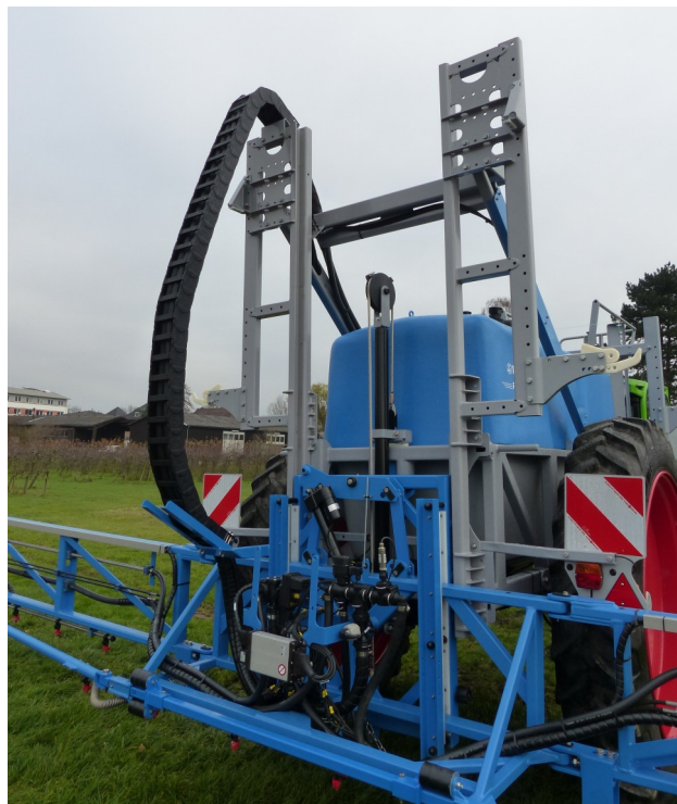
Fig.3: Steel boom with vertical lift.
