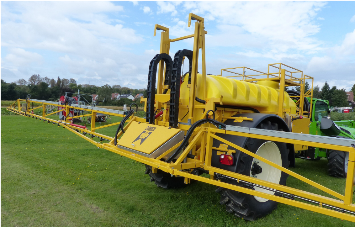
Fig.4: Rear view with boom and boom lift for the lateral folding boom.
