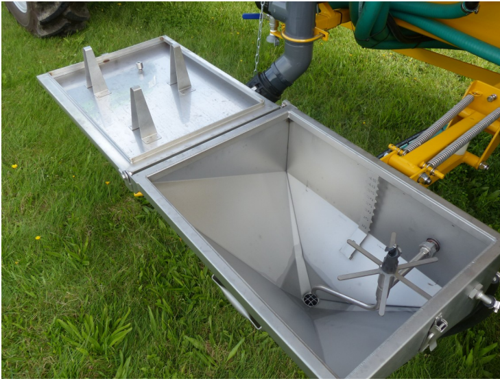
Fig.6: Stainless steel induction bowl with contents indicator and rotating nozzle for can rinsing.
