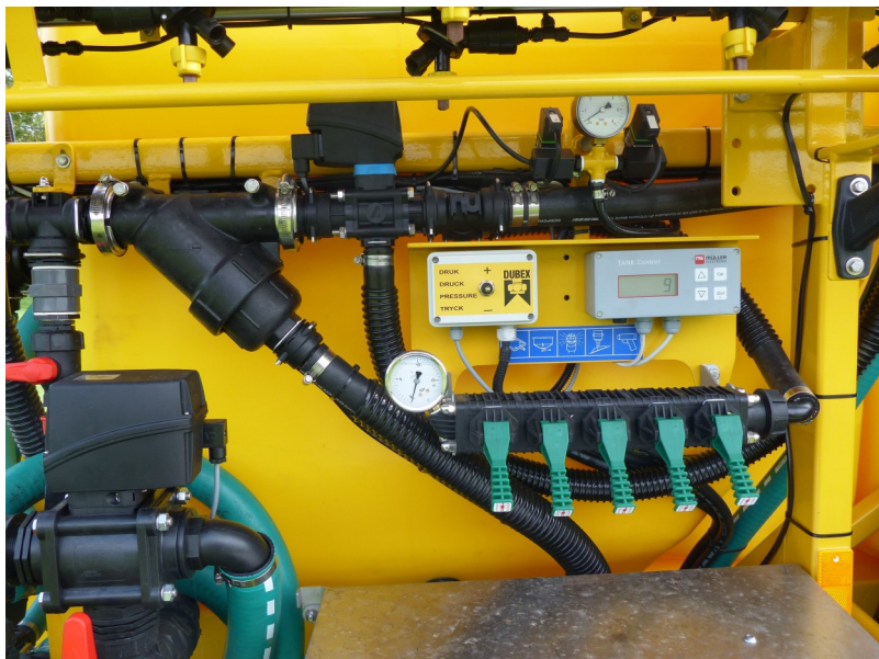
Fig.5: Control center on the left sprayer side.
