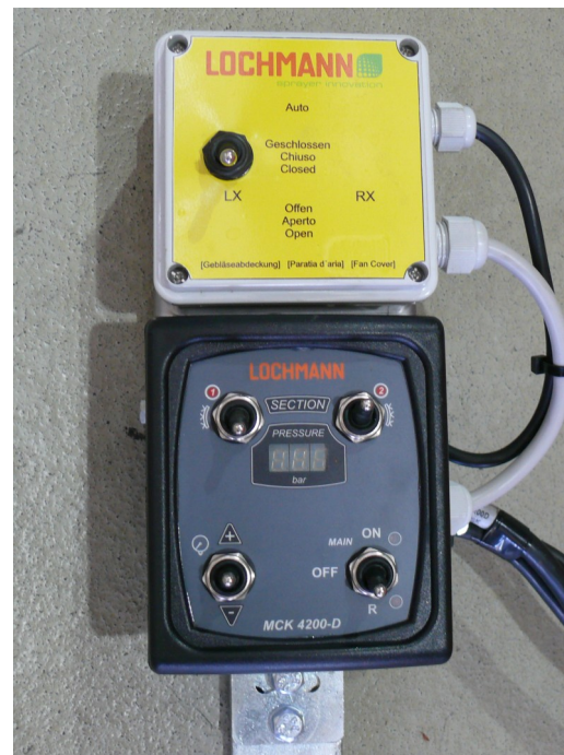
Fig.5: Switchbox with pressure gauge (below). (Above) optional switchbox for air cover shield.
