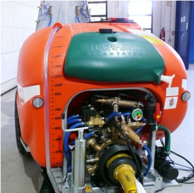
Fig.4: PTO driven pump and tank with contents indicator.
