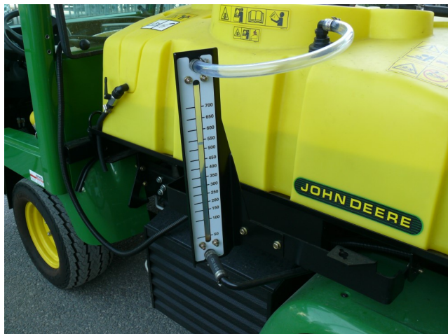
Fig.3: Tube (ball) tank contents indicator, with scales to the front and to the rear.
