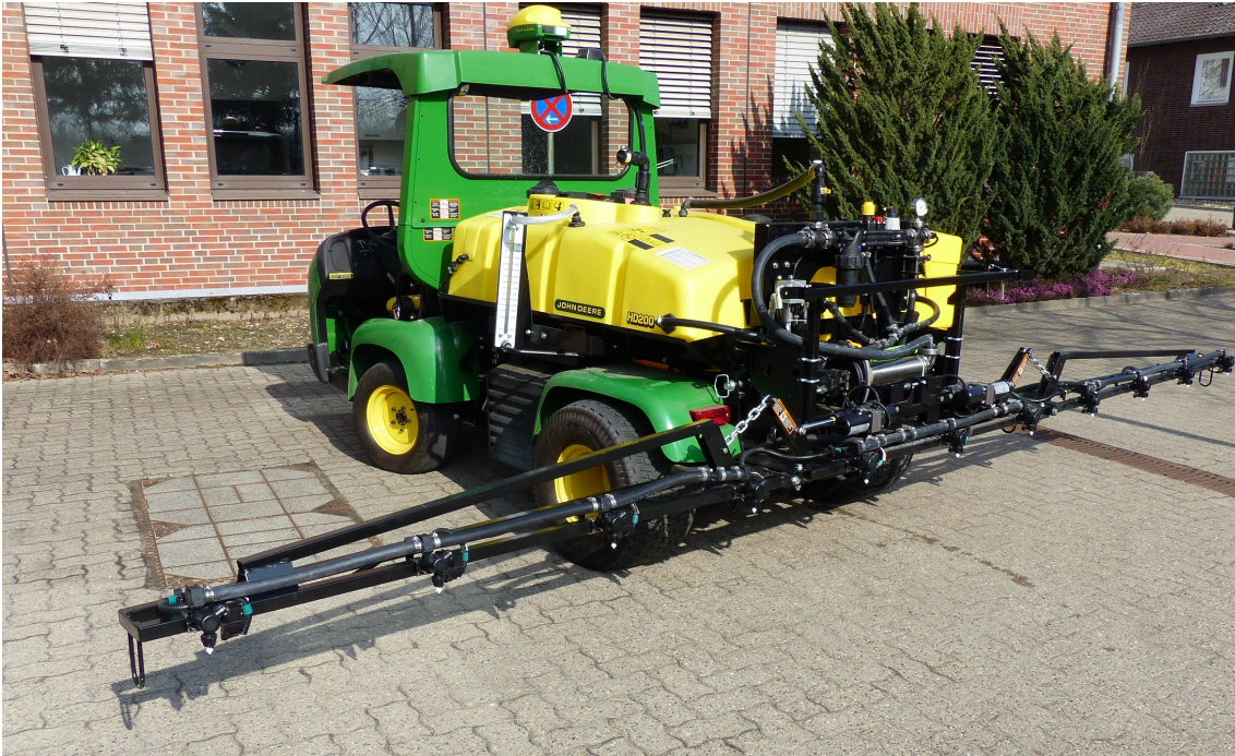
Fig.2: Left sprayer side, with new designed tank contents indicator and receiver of the GPS positioning system „StarFire 6000“ on the roof (optional, not tested).
