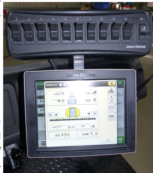
Fig.5: Spray computer and switch box.
