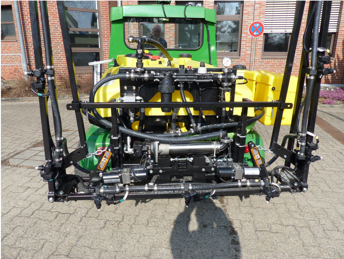
Fig.4: Rear view of the sprayer with the pressure regulation and filter unit.
