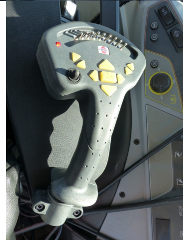
Fig.6/7/8: Terminal „HC 8600“ and switch box „SetBox“ or joystick mounted in the driver's cabin for displaying and controlling the sprayer functions.
