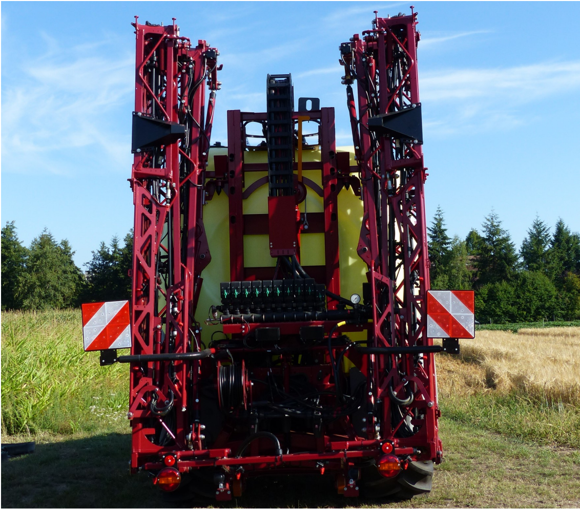
Fig.2: Rear view of the sprayer with boom package and the boom lift.
