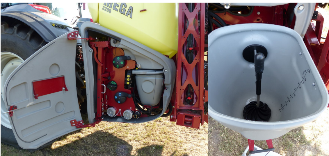
Fig.4/5: Left sprayer side with control centre and induction bowl.
