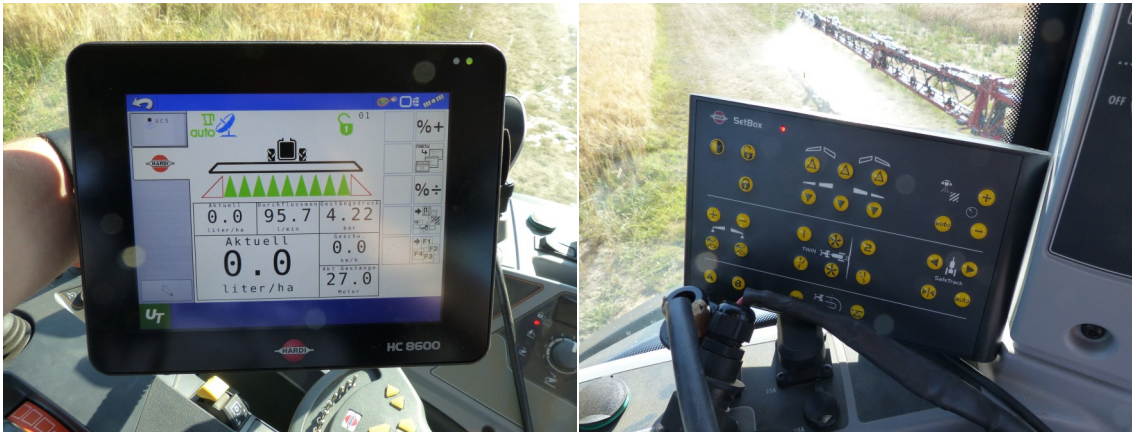
Fig.6/7/8: Terminal „HC 8600“ and switch box „SetBox“ or joystick mounted in the driver's cabin for displaying and controlling the sprayer functions.
