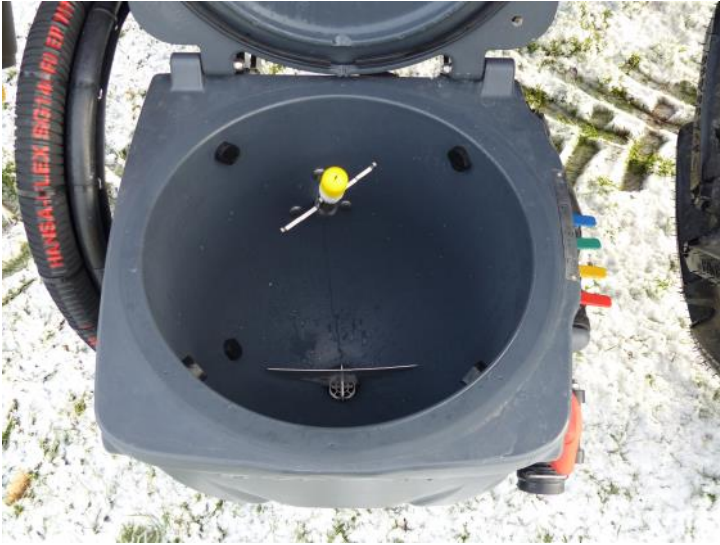
Fig.6: Polyethylene induction bowl with wall nozzles and rotating nozzle.
