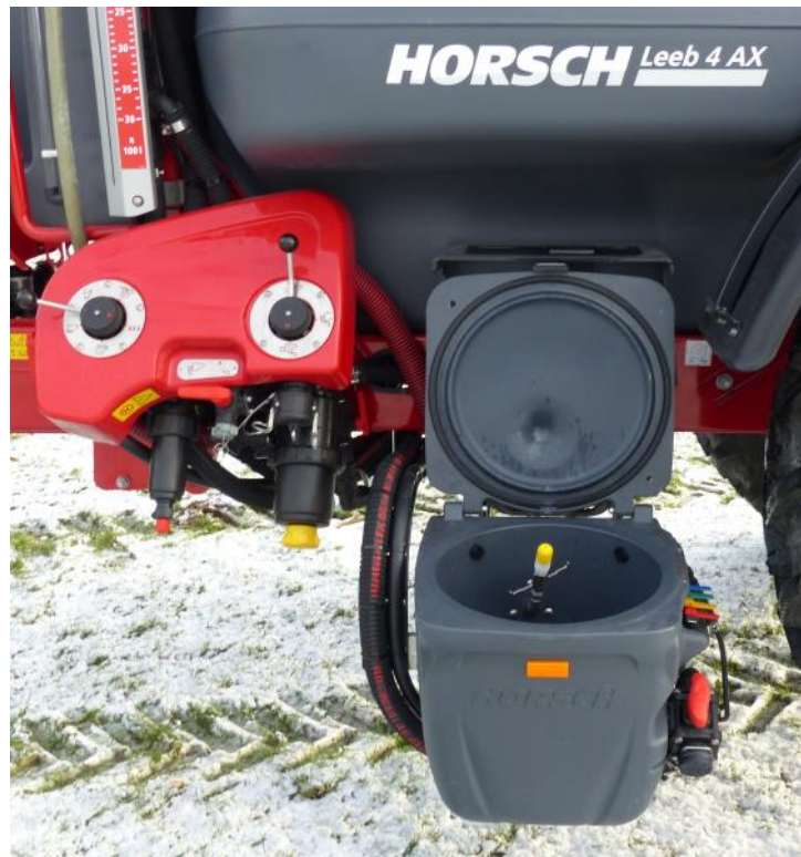
Fig.5: Left sprayer side with induction bowl, control center with filling connections and hand wash tank.
