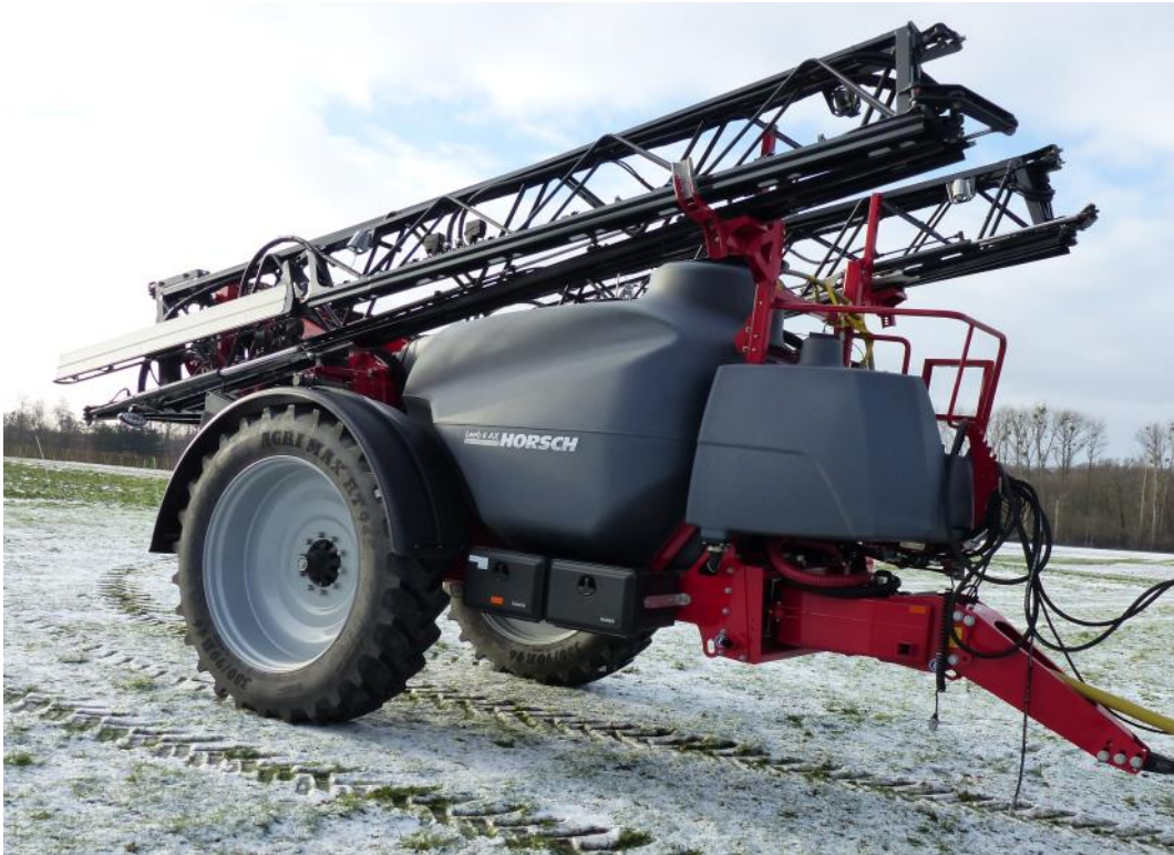
Fig.2: View of the right sprayer side with folded boom, storage compartment and wash water tank (over drawbar).
