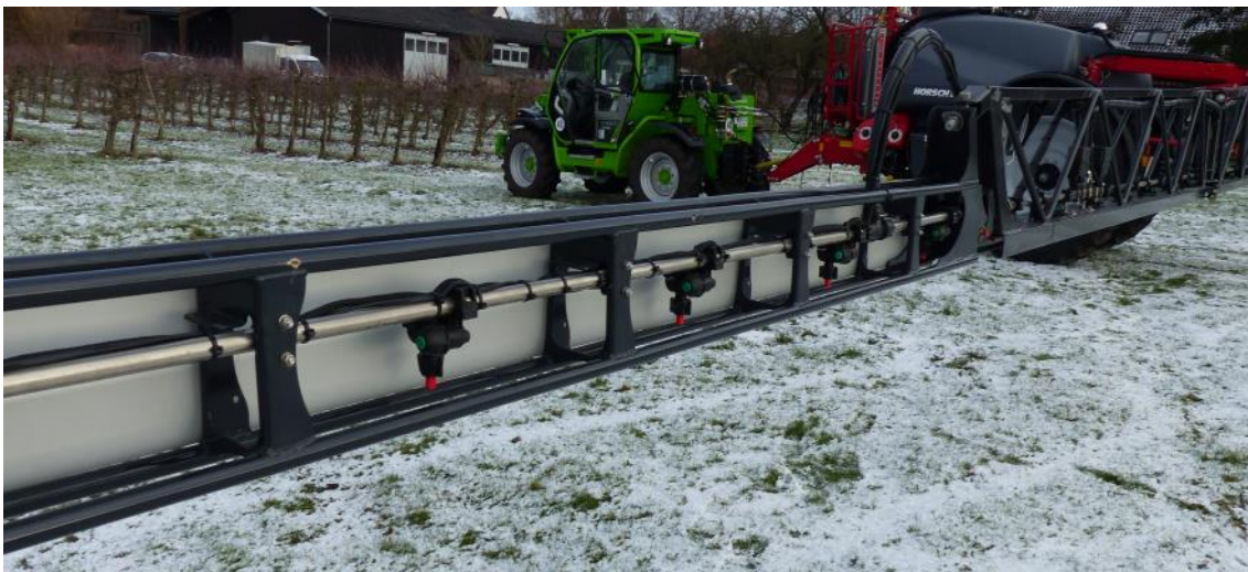
Fig.3: Outer boom section with well protected nozzles and obstacle give away function.
