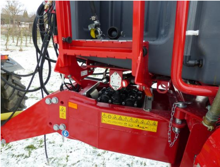
Fig.4: Steering drawbar with piston diaphragm pump. Blocking of steering function by bolt (right).
