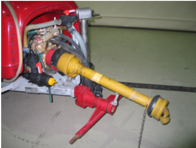
Fig.4: Front side with draw bar, pump, suction filter and front tank contents indicator
