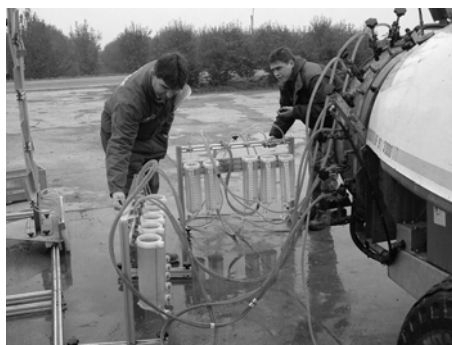
A – Measurement of tree crop sprayer nozzles flow rate
