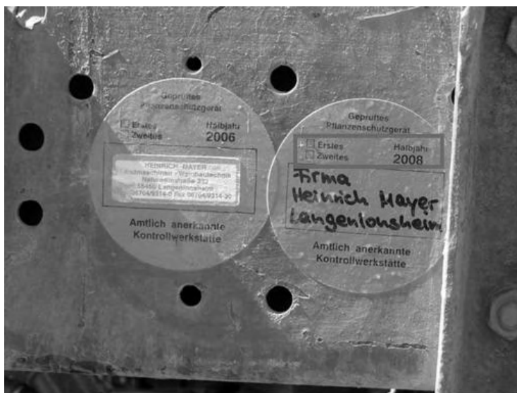
Figure4 Official stickers on the TPL demonstrate the mechanical workshop/ test operator and expiry date (second half-year 2006 and 2008 respectively). The colour of the sticker changes annually.
