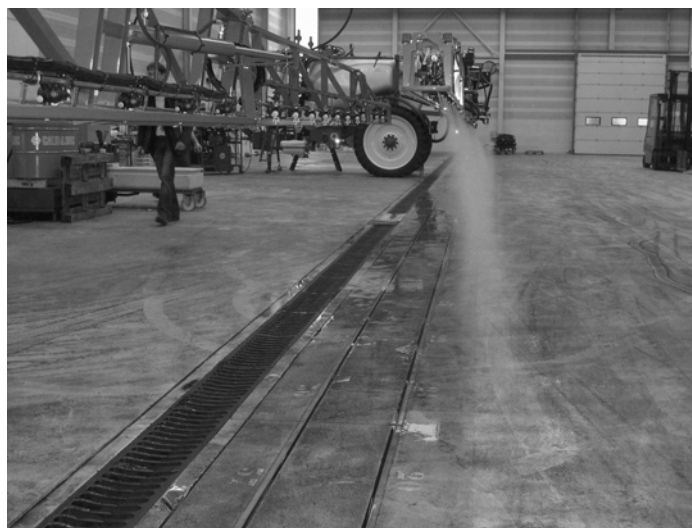
Figure 3 Inspection of brand new sprayers by built in spray scanner at John Deere Company
