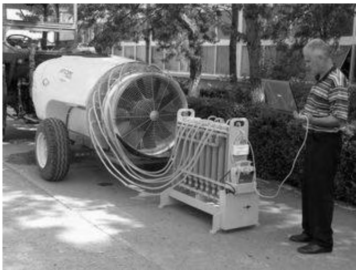
Figure 5 Testing the functional parameters of an air-assisted sprayer ATOM 1000, with the help of the stand built
