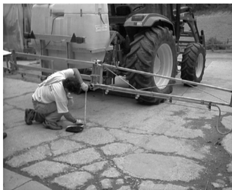
D – Checking of boom sprayer trim
