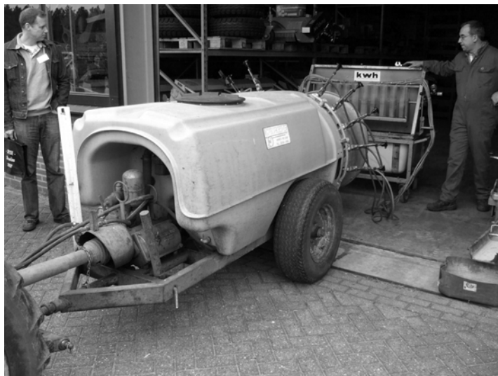
Figure 2 Determination of the nozzle output of a orchard sprayer at Coenders Company in the Netherlands
