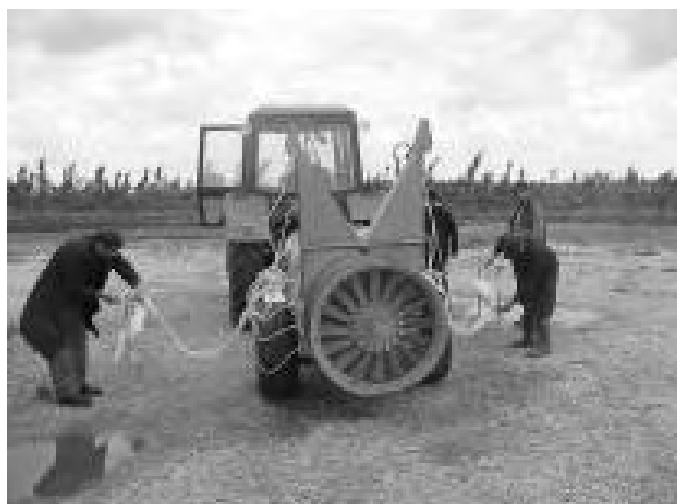
Figure 3 Measuring nozzle flow rate
