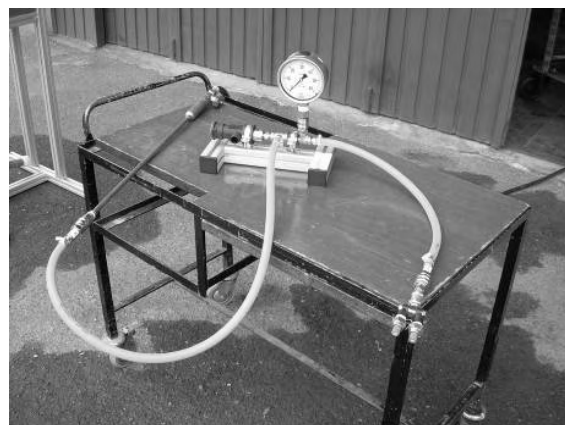
Figure 3 Prototype of test bench to assess pressure drop for spray lances.
