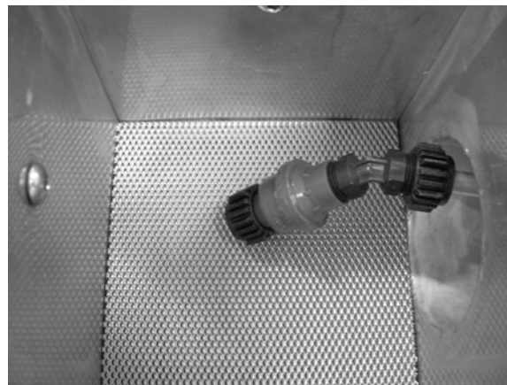
Figure 2 Detail of internal hopper for spray lance introduction
