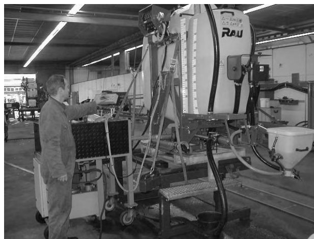
Figure 1 Inspection of a new sprayer comprises pump capacity, pulsations, leakages, safety valve and kinks
