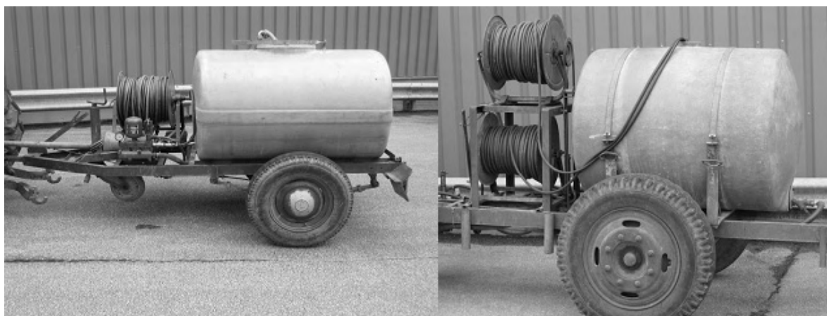
Figure1 Typical tank-pump-lance (TPL) units, with one and two hose reels
