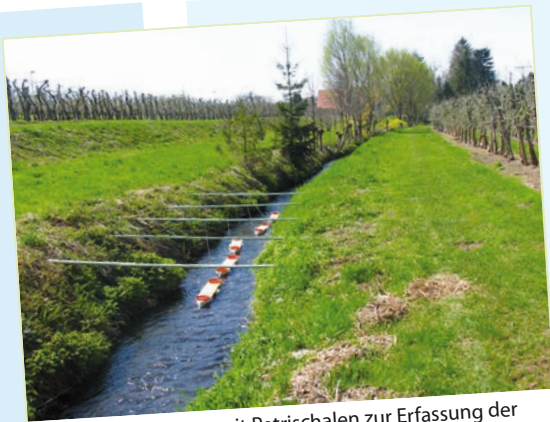
Fig. 5: Floater with Petri dishes to collect deposits of active substances
