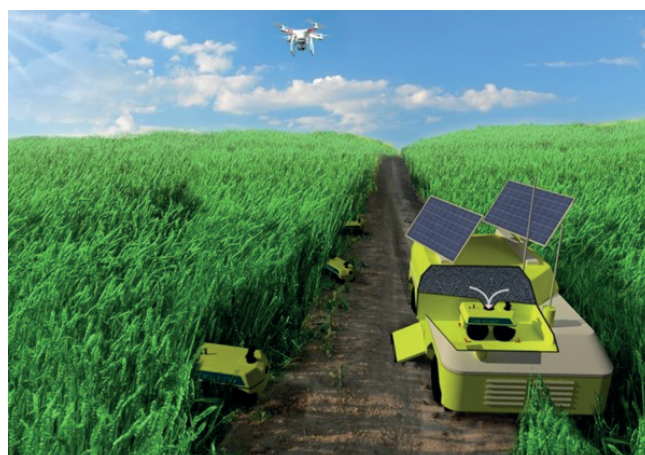
Fig. 4. Field station for the CareRowBot concept. At the field station the robots get refilled with required agents and batteries get exchanged. Photo: TU Braunschweig/Thünen-Institut/Julius Kühn-Institut and anko_ter – https://de.fotolia.com/ (modified from original)
