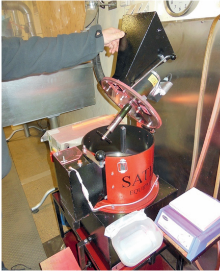
4. Batch seed treatment principle. Mixing chamber (rotating drum, cone with funnel for manual dosing and introduction of PPP (Photo: JKI)
