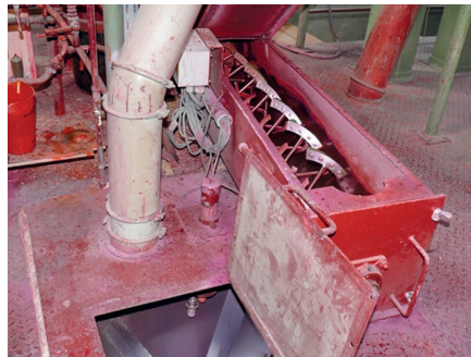
2. Continuous treatment: stationary equipment for cereals: Rotary atomizer followed by mixing auger in mixing chamber (Photos: H.-J. Osteroth, JKI)
