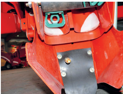
7. Mobile spraying on seeds: On potato-planter between hopper and soil (Photo: H.-J. Osteroth, JKI)
