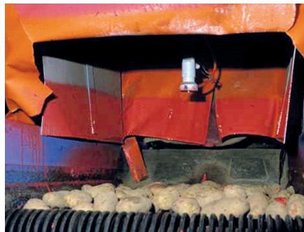
3. Continuous process; Semistationary equipment for treatment of potatoes, transport conveyer with rotary atomizer under hood (Photos: E Nilsson, Visavi Sweden. The photos are allowed for the use in this Spise Advice only!)
