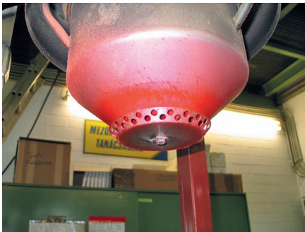
2. Continuous treatment: stationary equipment for cereals: Rotary atomizer followed by mixing auger in mixing chamber (Photos: H.-J. Osteroth, JKI)
