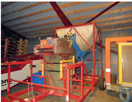
3. Continuous process; Semistationary equipment for treatment of potatoes, transport conveyer with rotary atomizer under hood (Photos: E Nilsson, Visavi Sweden. The photos are allowed for the use in this Spise Advice only!)
