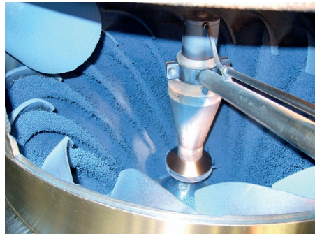
6. Batch treatment: Oil seed rape seeds with introduction of PPP via pump to rotating disc atomizer (Photo: H.-J. Osteroth, JKI)
