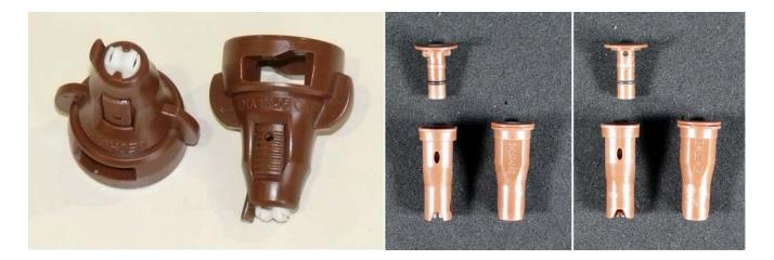
Mixed nozzle assembly comprising of Lechler IDTA 120-05 C (Certification number G 2018) and 6 x nozzle Lechler ID-120-05 POM (Certification number G 1966) or 6 x nozzle Lechler ID-120-05 C (Certification number G 1973) used in the area behind the sprayer to prevent the contamination of sprayer parts
