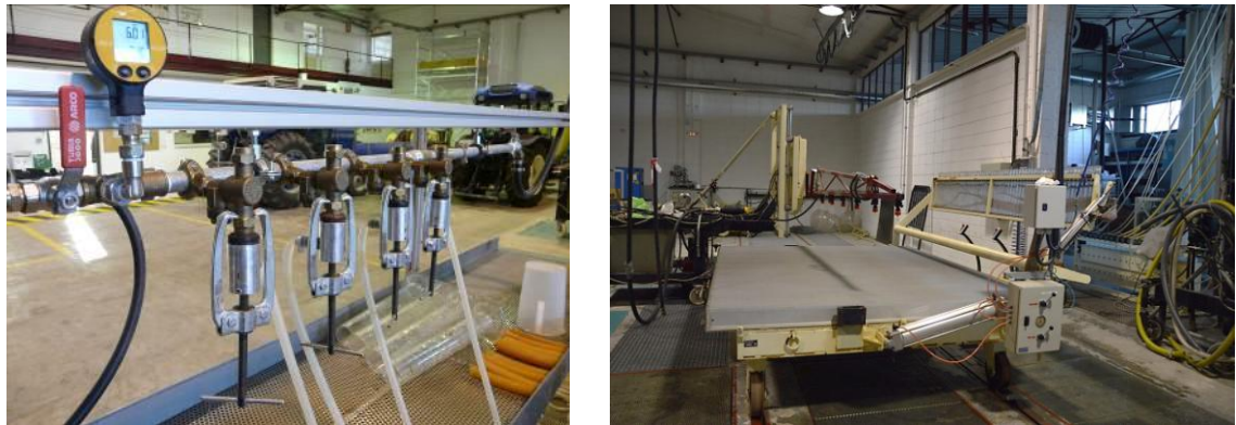
Figure 1. Water-tight adaptors for the measurement of the nozzle flow rate (left) and horizontal patternator for the measurement of the transverse distribution in boom sprayers.
