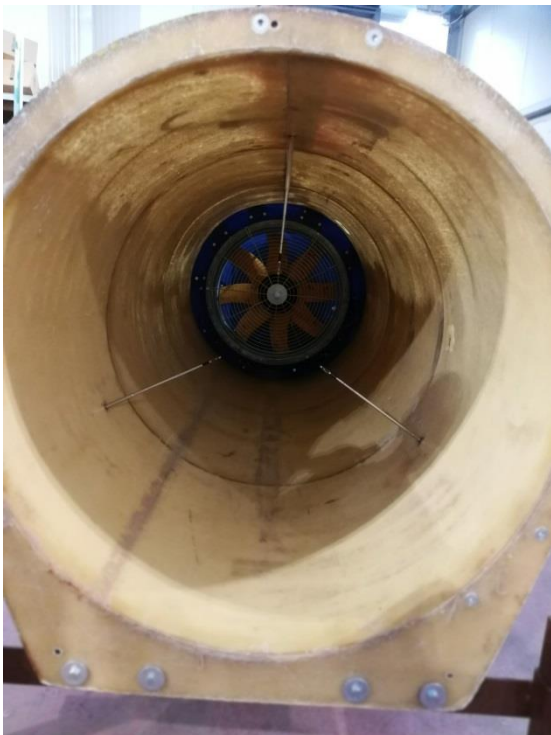
Figure 2: Measuring pipe of airflow at the intake
