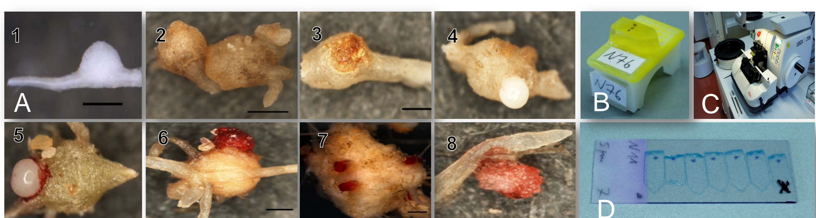
Fig. 3 Classification of gall specimens (A); embedding of galls in epoxy resin (B); sections of a specimen (C,D).
