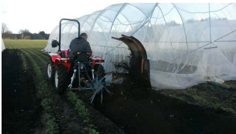
Photo 2 Hilling up soil by tractor with a modified ridge hilling machine
