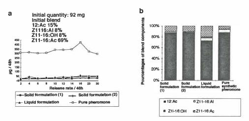
Figure 1 Results of effluvia collections: a) release rate of solid and liquid sprayable formulations; b) quality of the blend released
