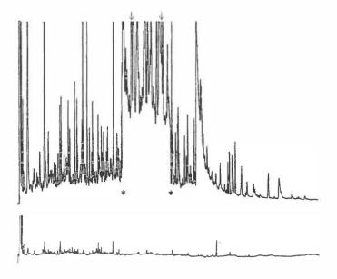
Figure 2 Gas chromatogram of 2.5 m<sup>3</sup> orchard air sampled during 2.5 hr on a Tenax filter. First arrow: internal standard (10 ng 13:OH); second arrow: codlemone. Asterisks indicate a change in signal amplification (attenuation)
