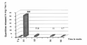
Figure 3 Quantity of pheromone released in the field from solid sprayable formulation of pheromone. Results were obtained by complete extraction. During 8 weeks 64.1 g/ha were released, 35.9 g/ha remained in solid formulation
