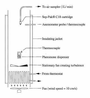
Figure 1 Apparatus to determine release rates of mating disruption dispensers, adapted from Pop et al. (1993)
