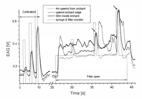
Figure 4 EAG signals recorded at different positions in the orchard. The response peaks to the calibration stimuli remain at the same absolute height; but the traces between these stimuli show strong variations, resulting from pheromone-loaded air packets arriving at the probe
