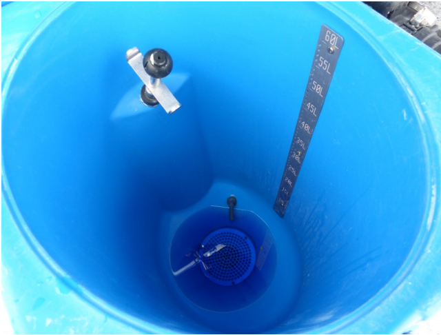
Fig.6: Induction bowl with contents indicator and rotating nozzle for can cleaning.
