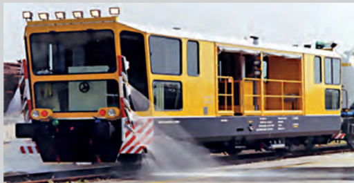
Fig. 2 – Example of special trains designed and built specifically for weed control on the railways used in Italy (Technical Services S.r.l., 00013 Fonte Nuova (RM)).
