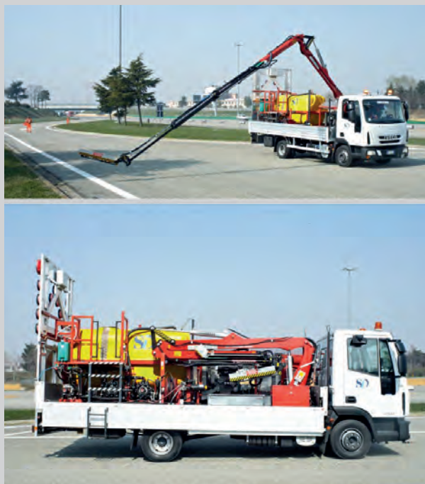
Fig. 5 – Example of special truck equipped with weed control system (Photo Sid Ambiente srl).
