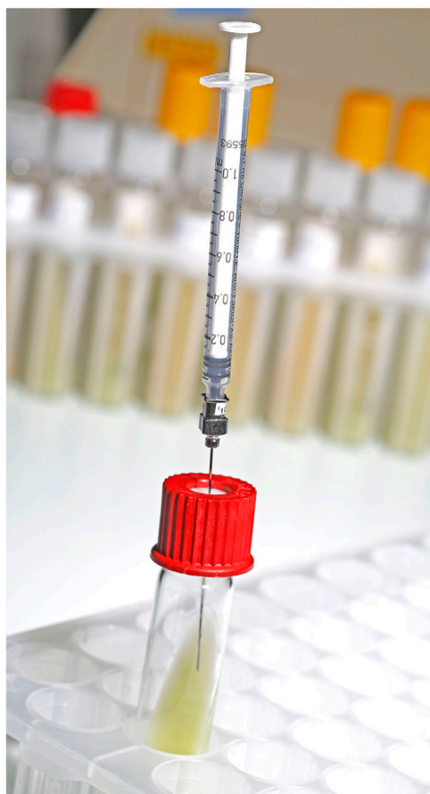
Figure 2. Experimental set up for sampling of headspace above culture media. Photo: FLI (W Maginot).
