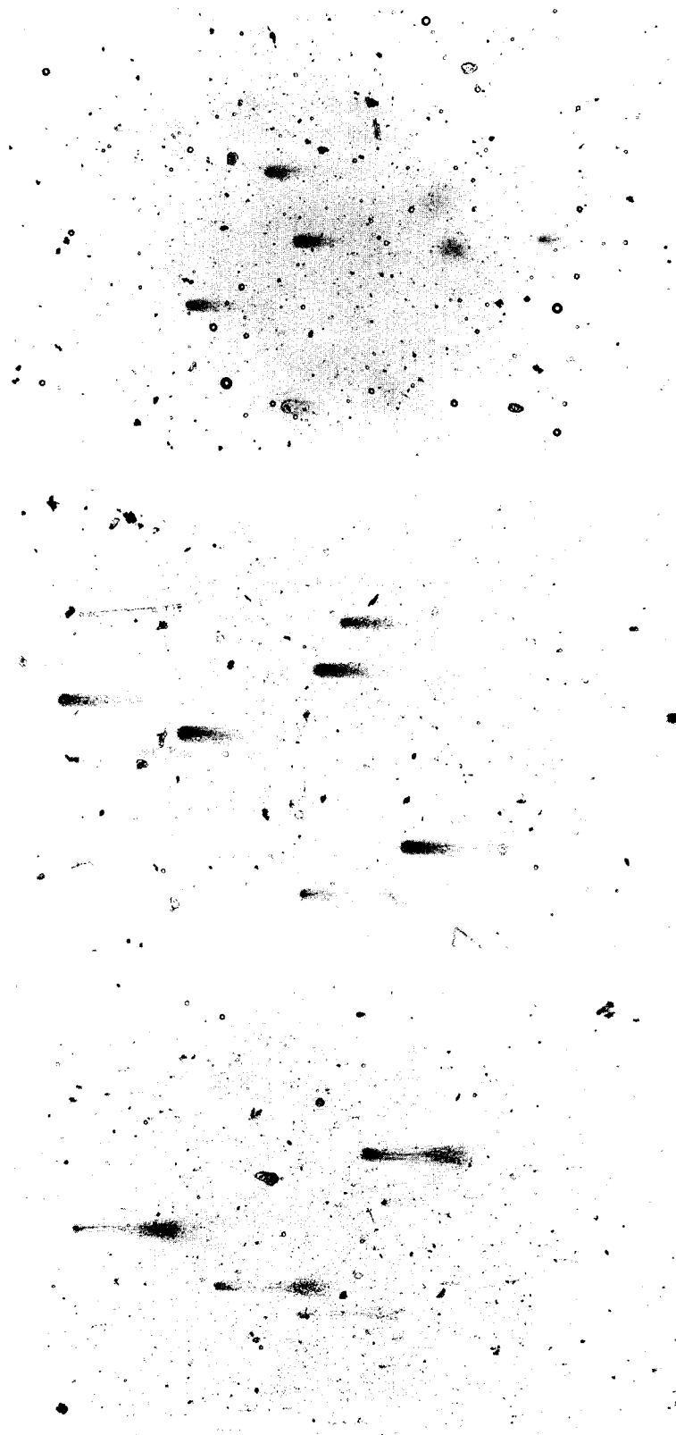
Fig. 1. Microgel electrophoresis of cells from grapefruit seeds; silver staining; anode to the right; radiation dose from top to bottom: 0, 0.2 and 0.5 kGy.
