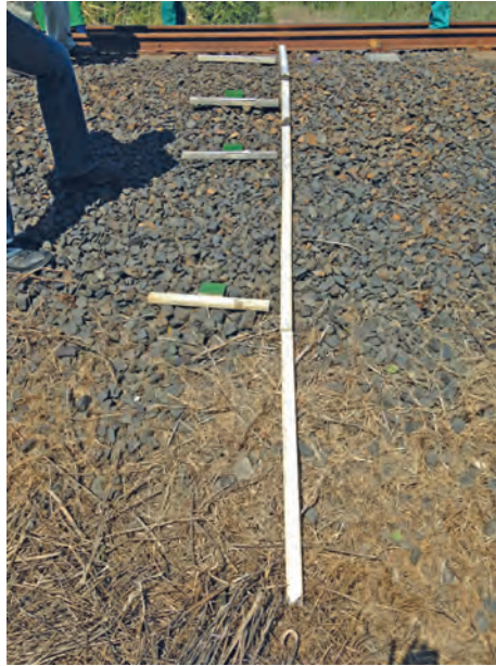
Fig. 6. Testing the lateral distribution of the spray train with filter paper. (Phot. Wegener).
