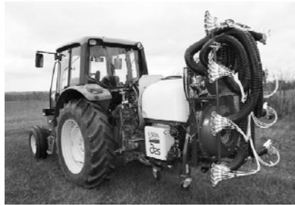
Figure 1. Newly developed automated variable-rate, air-assisted precision sprayer
