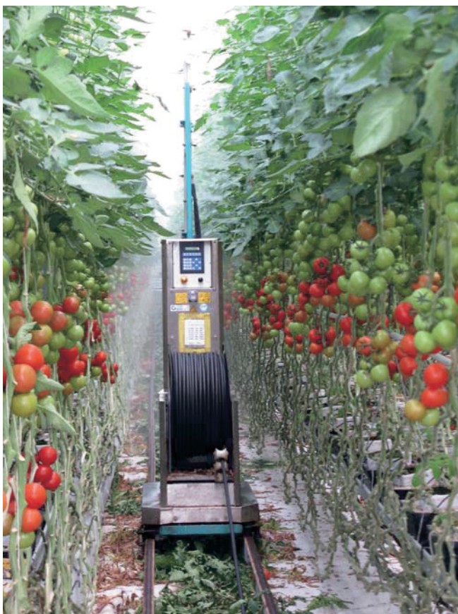
Fig. 1. Application of XenTari® with a half automatic application robot (Meto, Berghortimotive) (left), and with reduced numbers of opened nozzles (right).
