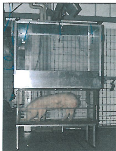
Figure 1: Helium stunning design, longitudinal side; experimental animal already driven into the cage, shortly before the stunning cycle began
