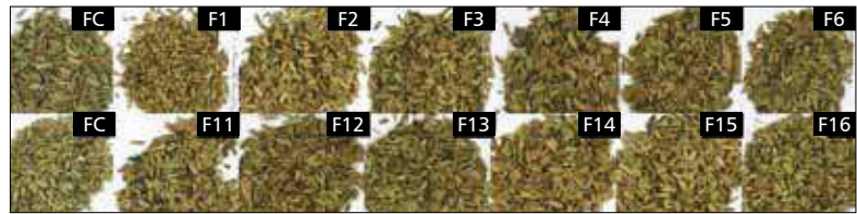
Fig. 2: Fennel before and after mechanical saturated steam decontamination. FC = Control, F1 – F6 = single treatment with saturated steam, F11 – F16 = double treatment with saturated steam. For details of the treatment see Tab. 1 .
