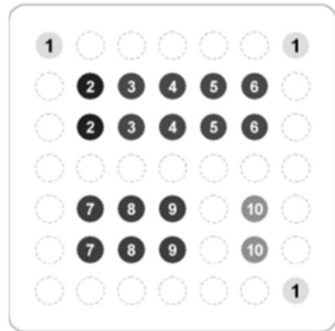
Fig. 1. Arrangement of the probes of LCD-microarray system B.T.A. 1.0 (Chipron GmbH, Berlin, Germany) designed for this study: 1 hybridization-control, 2 Piroplasmidae , 3 Babesia (B.) bovis , 4 B. divergens , 5 B. bigemina , 6 B. major , 7 Theileria (T.) mutans , 8 T. annulata , 9 T. parva , 10 not used.
